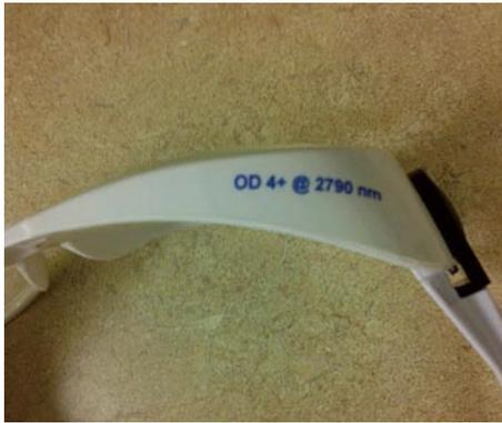
Figure 3 Optical density engraved on laser safety eyewear.
