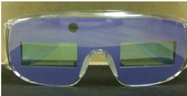
Figure 5 Shutter glasses used for intense pulsed light.
