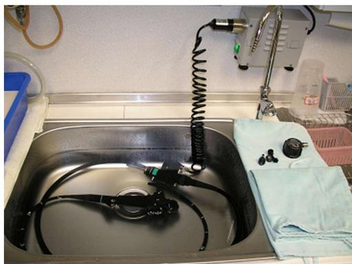
**Figure 2** A manual leak test is conducted to examine any damage in and out of the gastrointestinal endoscope. It is very important to protect the endoscope from damage from the cleansing solution. No air bubbles should appear after attaching the water-resistant cap.
