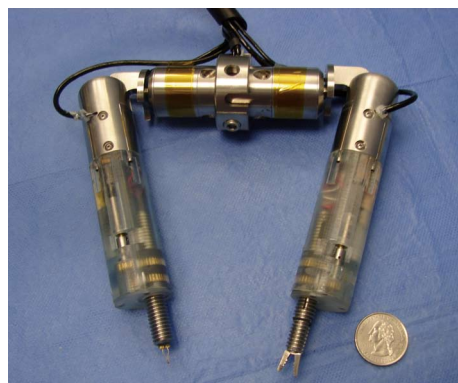
Figure 4 Prototype in vivo dexterous robot with grasper and cautery end effector arms.
