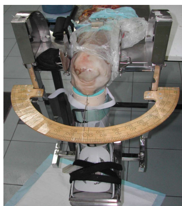
Figure 2 Knee rotation jig with specimen mounted with nail through tibial tuberosity and skin pointer in place.
