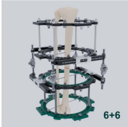
Figure 3 Compression-distraction apparatus for external fixation featuring six degrees of freedom[47]. Citation: Matsukatov FA. Compression-distraction apparatus for external fixation and method of closed reduction of bone and bone fragments. Euroasian patent register. https://old.eapo.org/en/patents/reestr/patent.php?id=45163 . Copyright ©The Author(s) 2023 (Supplementary material).
