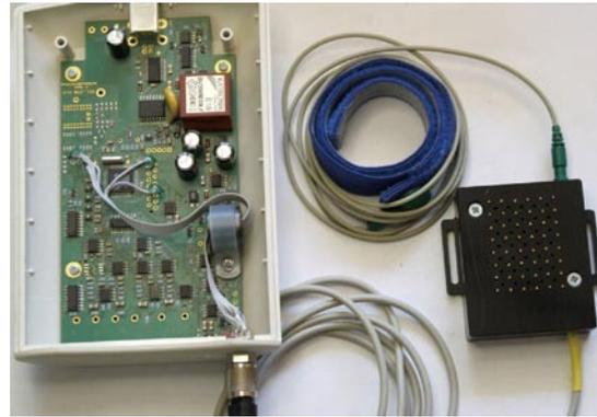
Figure 1 Measurement system for electrodermal mapping (modified from<sup>[14,15]</sup>).
